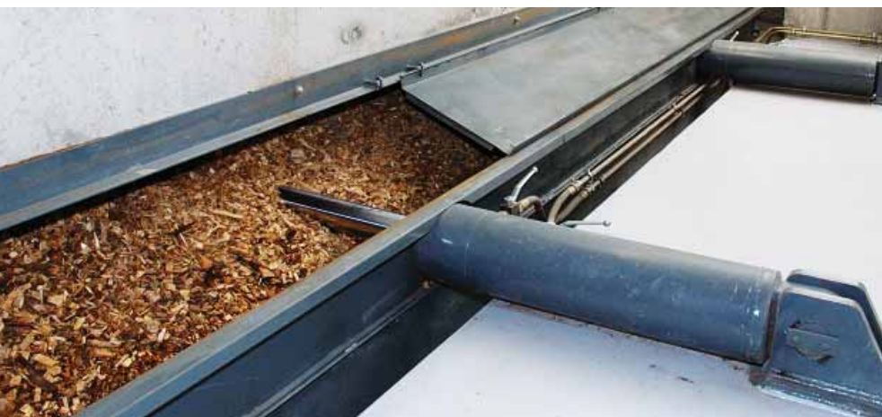
Walking floor installation
